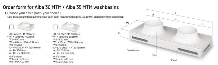
$^*$  W1 = Recommended (min-max) size when the mixer from the wall
