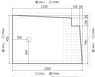
The dimensions of the drawing are:  $\bigcirc$  DIMENSIONS FOR THE WALL  $$\boxtimes$$  DIMENSIONS FOR THE SHOWER TRAY
