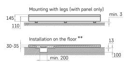
stst 3 mm thick polypropylene must be laid between the shower tray and the surface
